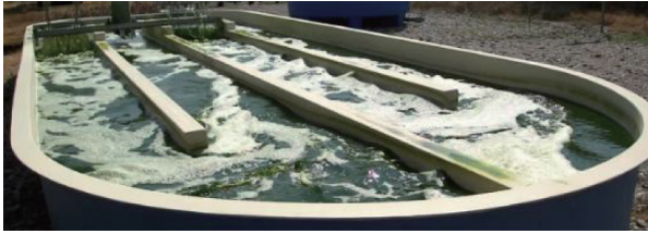
Cheng-Kung Univ. 20 t Raceway Pond for Microalgae Cultivation
